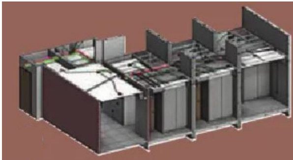
Figure 21: MEP systems integrated into PPVC modules
